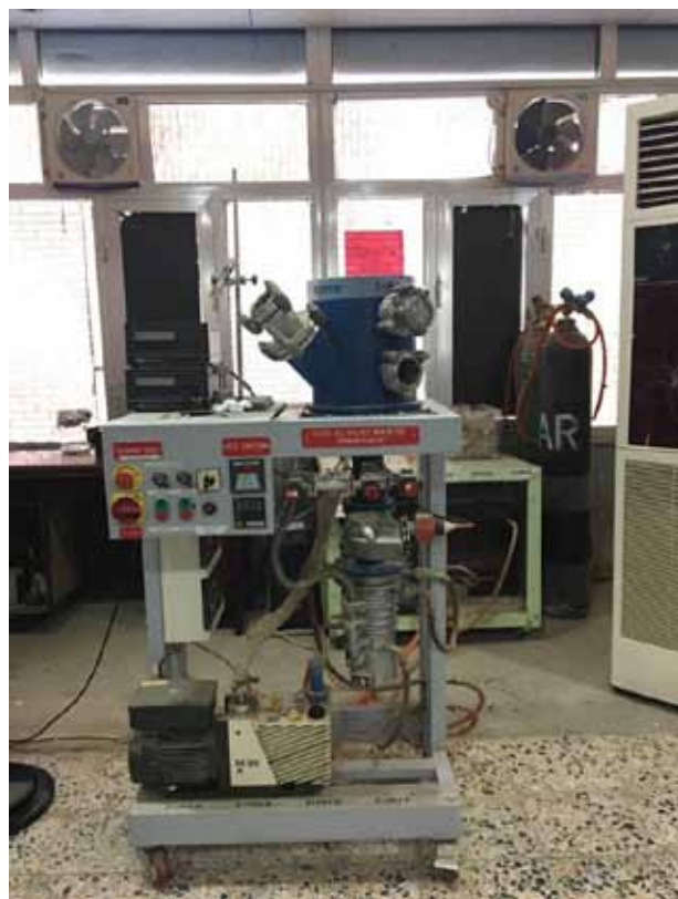
Fig(3): Pulse laser deposition system.
