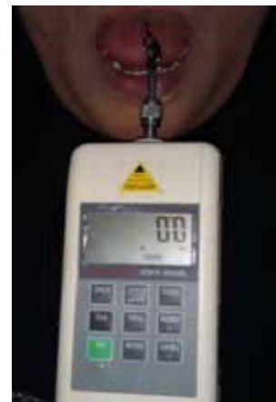
Fig (3): Digital force gauge device attached to the maxillary partial denture
